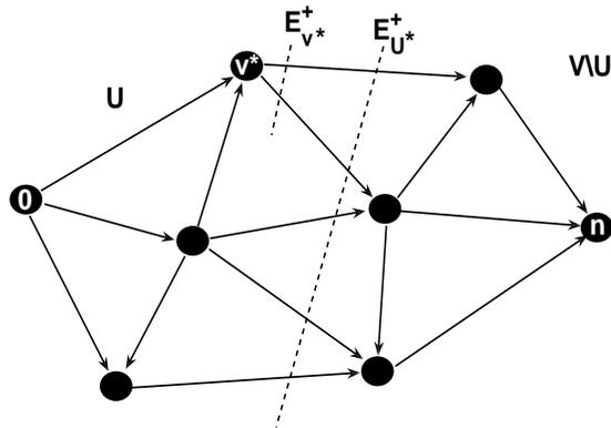
Fig. 2. Comparison between a node-cut and a min-cut of a flow network.
