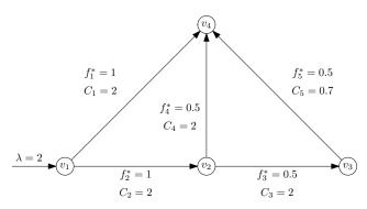
Fig. 2: A single-commodity network. The minimum residual capacity 0.2 is achieved at node  $v_3$ . Hence, under any perturbation of magnitude smaller than 0.2 the network is still be able to transfer the external inflow  $\lambda_{v_1}$  to the destination node  $v_4$ .
