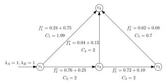
(b) The same network when edge  $e_1$ 's capacity is slightly decreased. Now the inflow to link  $e_5$  is larger than its capacity, and hence the network is not able to handle the flow demands.
