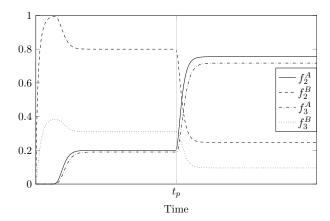
Fig. 5: The time evolution of flows on link 2 and 3. At time  $t=t_p$  a perturbation occurs and causes the flow  $f_3$  on link 3 to exceed the capacity of link 5. As a consequence, the density on link 5 grows unbounded and the network loses the property of being fully transferring.
