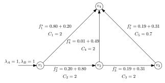
(a) Equilibrium flows for a simple network. All flows are less than edges capacities, so that the network is able to fully transfer the external inflows  $\lambda_A, \lambda_B$  to their destinations, node  $v_4$ .
