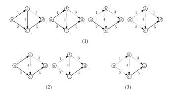
Figure 4. Sequences of link failures under finite buffer capacities using routing matrices analogous to those in Sec. II. Only link 3 is perturbed, with  $C_3 - \tilde{C}_3$  equal to  $\nu^{(1)}(0) = 1/3$ ,  $\nu^{(2)}(0) = 2/3$ , and  $\nu^{(3)}(0) = 1$ , respectively.
