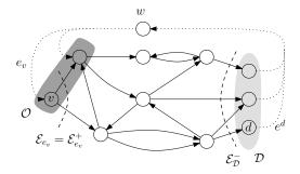
Figure 6. A network  $\mathcal{G}$  and the augmented network  $\mathcal{G}^a$ . The links in  $\mathcal{E}_{\mathcal{D}}^-$  and  $\mathcal{E}_{\mathcal{D}}^+$ , added in  $\mathcal{G}^a$ , are shown in dotted line. The set of origins and the set of destinations are shown in dark grey and light grey, respectively.
