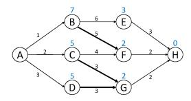
Now the optimal "cost-to-go" at "E", "F" and "G" can be used to get the optimal "cost-to-go" at "B", "C" and "D".
