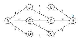
We proceed with backward induction. Once the final node is reached the remaining cost is 0.
