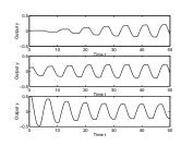
$Frequency\ and\ amplitude\ independent\ of\ initial\ conditions!$ Several systems use the existence of such a phenomenon
