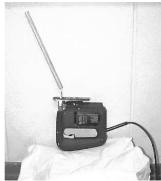
Figure 1.11 The inverted pendulum on an electric hand-saw in Exercise 1.16
