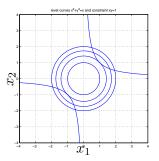
Level curves for constant  $g_1$  and the constraint  $g_2 = 0$ , repectively.
