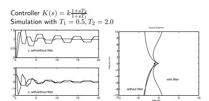
No limit cycle, oscillation removed!
