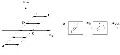
Idea: Let  $x_{\rm in}$  jump  $\pm 2D$  when  $\dot{x}_{\rm out}$  should change sign. Works if the backlash is directly on the system input!
