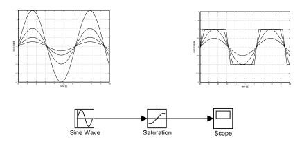
The "effective gain" ( the ratio  $\frac{\mathrm{sat}(A\sin\omega t)}{A\sin\omega t}$ ) varies with the input signal amplitude A.
