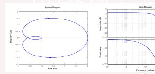
Since the third describing function fulfills that  $-\frac{1}{N(2)}=-\frac{1}{2}$  and  $G(i\omega_o)\approx -0.6$ , we understand that we have **two** intersections. The first intersection occurs when  $A\approx 1.8$  and the second intersection occurs when  $A\approx 4.5$ .
