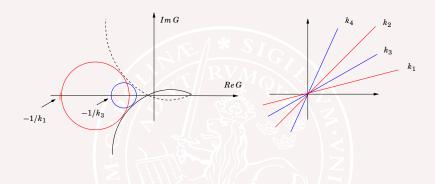
In the example above, the circle criterion can guarantee absolute stability for a nonlinearity which is bounded to **either** the sector  $[k_1, k_2]$  **or**  $[k_3, k_4]$  or in many other sectors, but NOT for a nonlinearity which is allowed to have a full variation within the sector  $[k_1, k_4]$ .
