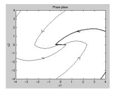
The dynamics along the sliding set in  $\sigma(x) = 0$  can also be obtained by finding  $u = u_{eq} \in [-1, 1]$  such that  $\dot{\sigma}(x) = 0$ .
