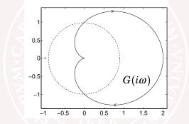
The Nyquist Theorem proves stability when  $K \in [0, \infty)$ . The Small Gain Theorem proves stability when  $K \in [0, 1/2)$ .
