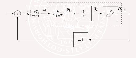
Controller  $K(s) = k \frac{1+sT_2}{1+sT_1}$ Simulation with  $T_1 = 0.5, T_2 = 2.0$
