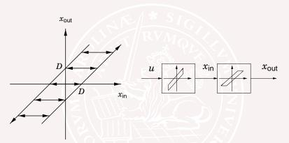
Idea: Let  $x_{in}$  jump  $\pm 2D$  when  $\dot{x}_{out}$  should change sign. Works if the backlash is directly on the system input!
