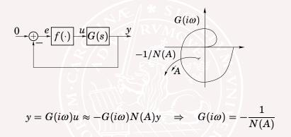
The intersections of  $G(i\omega)$  and -1/N(A) give  $\omega$  and A for possible limit cycles.
