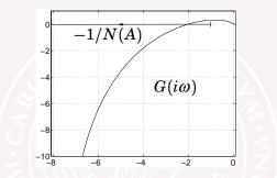
Introduce N(A) as an amplitude dependent gain-approximation of the nonlinearity  $f(\cdot)$ .
