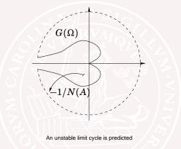
An intersection with amplitude  $A_0$  is unstable if  $A < A_0$  gives decreasing amplitude and  $A > A_0$  gives increasing.
