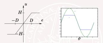
Let  $e(t) = A \sin \omega t = A \sin \phi$ . First set H = D. If  $A \le D$  then N(A) = 1, if A > D then for  $\phi \in (0, \pi)$
