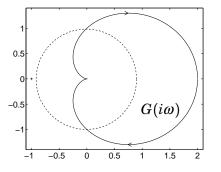
The Nyquist Theorem proves stability when  $K \in [0, \infty)$ . The Small Gain Theorem proves stability when  $K \in [0, 1/2)$ .
