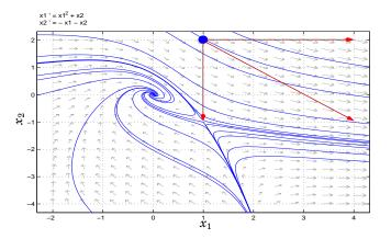
In the point  $(x_1, x_2) = (1, 2)$  the vector field is pointing in the direction  $(1^2 + 2, -1 - 2) = (3, -3)$ .
