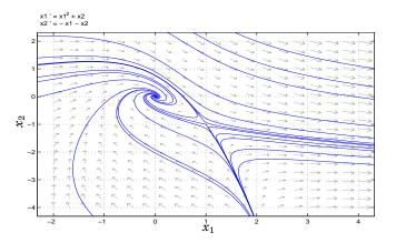
Flow-interpretation: To each point  $(x_1, x_2)$  in the plane there is an associated flow-direction  $\frac{dx}{dt} = f(x_1, x_2)$
