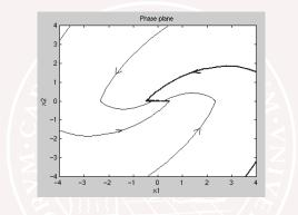
The dynamics along the sliding set in  $\sigma(x) = 0$  can also be obtained by finding  $u = u_{eq} \in [-1, 1]$  such that  $\dot{\sigma}(x) = 0$ .
