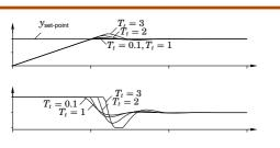
With very small  $T_t$  (large gain  $1/T_t$ ), spurious errors can saturate the output, which leads to accidental reset of the integrator. Too large  $T_t$  gives too slow reaction (little effect).
