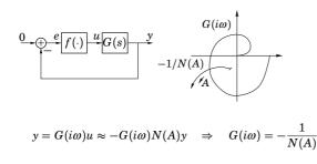
The intersections of  $G(i\omega)$  and -1/N(A) give  $\omega$  and A for possible limit cycles.
