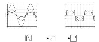
The "effective gain" (the ratio  $\frac{\operatorname{sat}(A\sin\omega t)}{A\sin\omega t}$ ) varies with the input signal amplitude *A*.
