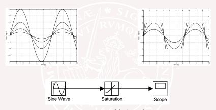
The "effective gain" ( the ratio  $\frac{\mathrm{sat}(A\sin\omega t)}{A\sin\omega t}$ ) varies with the input signal amplitude A.
