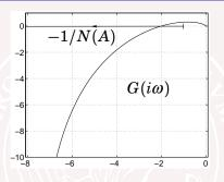
Introduce N(A) as an amplitude dependent gain-approximation of the nonlinearity  $f(\cdot)$ .
