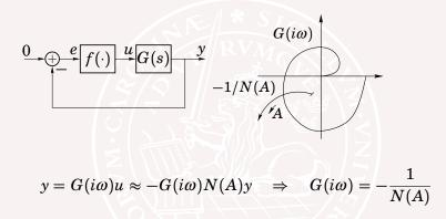
The intersections of  $G(i\omega)$  and -1/N(A) give  $\omega$  and A for possible limit cycles.
