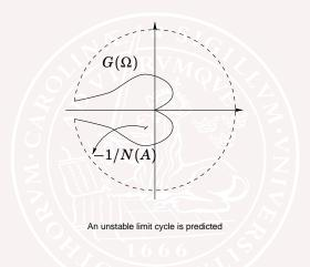
An intersection with amplitude  $A_0$  is unstable if  $A < A_0$  gives decreasing amplitude and  $A > A_0$  gives increasing.
