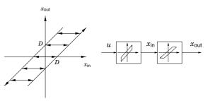
Idea: Let  $x_{\rm in}$  jump  $\pm 2D$  when  $\dot{x}_{\rm out}$  should change sign. Works if the backlash is directly on the system input!
