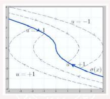
Combination of solution curves: Follow one parabola using maximum or minimum control signal until you hit the switch curve  $\sigma$ , switch to minimum/maximum control and then follow that parabola to the origin.
