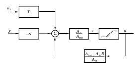
The freedom in  $A_n$  can be used to shape the response to errors due to saturation
