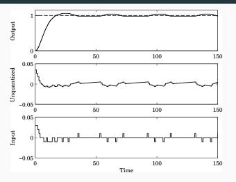
Limit cycle in process input with period 39 s, amplitude 0.01 (can be predicted with describing function analysis)
