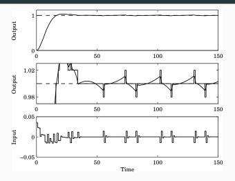
Limit cycle in process output with period 28 s, amplitude 0.01 (can be predicted with describing function analysis)
