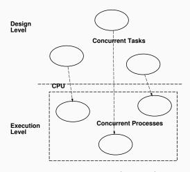
The CPU is shared between the processes (switches).
