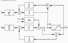
A change in a parameter when in stationarity should not result in a bump in the control signal.
