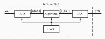
Controller G(s) is designed based on analog techniques
