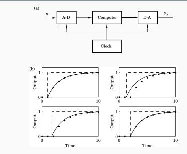
A sampler in direct combination with a ZOH device gives an average delay of h/2
