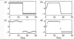
(a), (c):  $f_1 = 0.9$  Hz,  $f_N = 0.5$  Hz  $\Rightarrow f_{alias} = 0.1$  Hz
