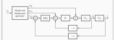
$\bullet$  The PID controller should have derivative weighting  $\gamma=1$
