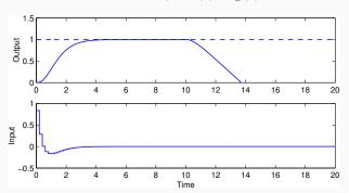
Does not work – the feedback term is needed to stabilize the process and handle the load disturbance
