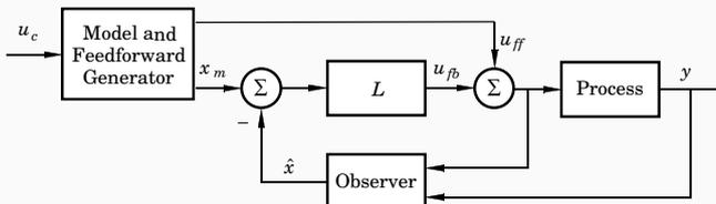
The model should generate a reference trajectory  $x_m$  for the process state  $x$  (one reference signal per state variable)
