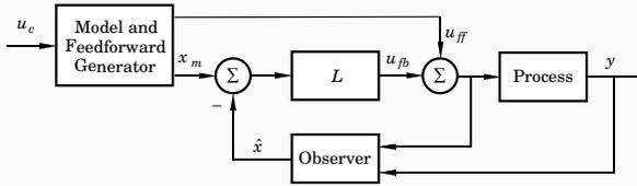
$u_{ff}$  and  $x_m$  do not have to come from linear filters but could be the result of solving an optimization problem, e.g.:
