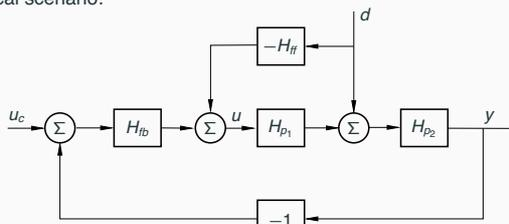
Pulse transfer function from measured disturbance  $d$  to output  $y$ :
