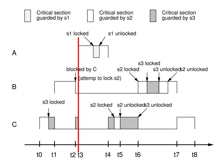
•  $t_3$ : A preempts C. Later is tries to lock  $s_1$  and succeeds (the priority of A is higher than the ceiling of  $s_3$ ).
