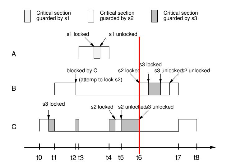
•  $t_6$ : C unlocks  $s_3$ , and gets back its basic priority. B preempts C, tries to lock  $s_2$  and succeeds. Then B locks  $s_3$ , unlocks  $s_3$  and unlocks  $s_2$
