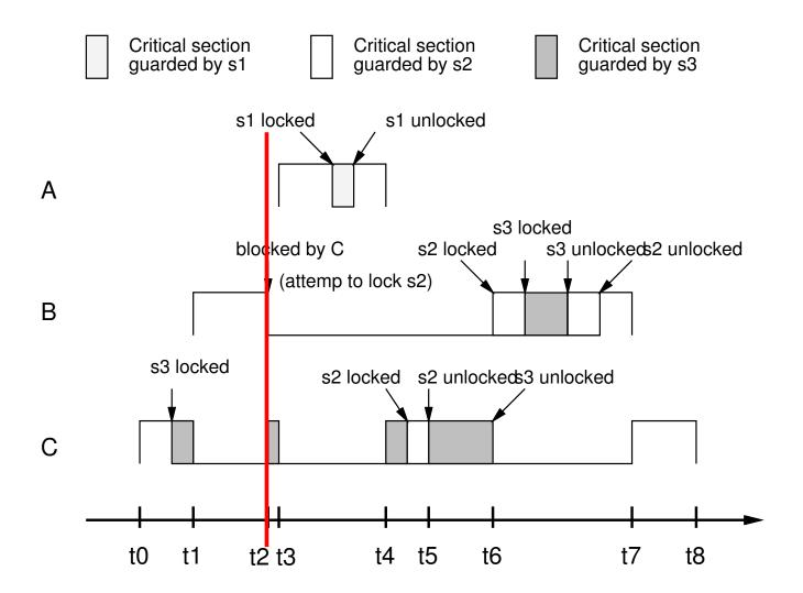
•  $t_2$ : B tries to lock  $s_2$ . B fails (the priority of B is not strictly higher than the ceiling of  $s_3$  that is held by C) and blocks on  $s_3$  (B is blocked by C). C inherits the priority of B.
