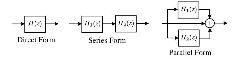
Try to balance the gain such that each subsystem has about the same amplification
