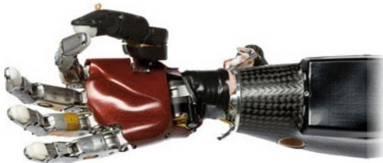
**Figure 1.1:** Robotic hand using 15 DC-motors to position 5 fingers independently. Having good models of the motors is crucial when developing a high-precision control system for the hand.
