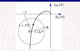
Closed loop stability with  $P(s) + \Delta(s)$  is guaranteed if nominal loop is stable and
