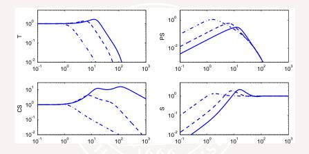
Gain curves of the Gang of Four for a heat conduction process with I (dash-dotted), PI (dashed) and PID (full) controllers.
