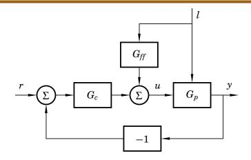
How to choose compensator  $G_{ff}(s)$ ? Depends on where disturbance l enters the system.
