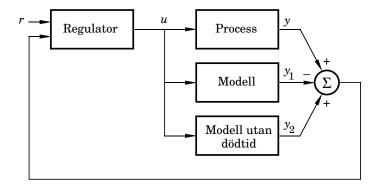
Controller designed after model without delay. Model must be:
