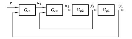
Secondary controller G<sub>c2</sub> controls y<sub>2</sub>
