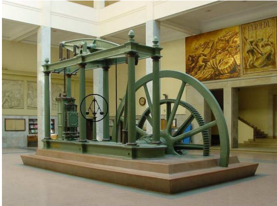
Watts steam engine (first from 1775)
