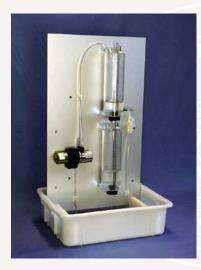
Control of the water level in the upper or lower tank
