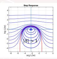
TAT: Explain the symmetry between the level curves of  $|T|=|\frac{L}{1+L}|$  and  $|S|=|\frac{1}{1+L}|$
