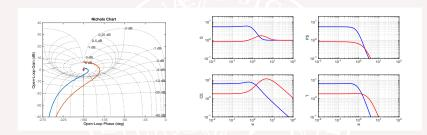
Better design: controller poles -2, -2, observer poles=-4, -4  $M_s=1.8(6.1)$ , phase margin  $\phi_m=36^\circ(9^\circ)$ ,  $\omega_{gc}=1.8(0.6)$  rad/s Note that higher controller gain is needed
