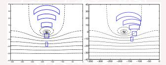
Closed loop system stable for all parameters.
