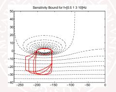
$$P(i\omega) = \frac{ka}{i\omega(i\omega + a)}, \quad k \in [1, 5], \quad a \in [1, 4]$$
