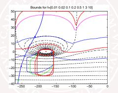
Low frequency gains is roughly right, but about 100 degrees more phase advance is needed around 0.5Hz
