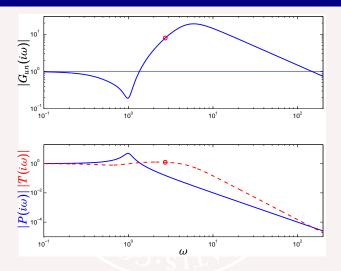
Notice that controller gain is high way beyond the gain crossover frequency marked with the red dots
