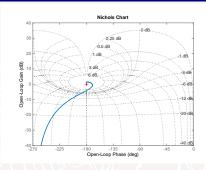
This is the state-feedback with Kalman filter design for the inverted pendulum  $G(s) = \frac{1}{s^2-1}$  in the basic course.
