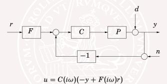
First design feedback  $C(i\omega)$  to reduce effects of uncertainty and disturbances, considering structure of process variations
