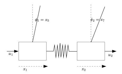
The process consists of two inverted pendulums mounted on movable carts. The carts are connected with a spring. The inputs are the forces on the two carts. The outputs are the cart positions and pendulum angles. The system hence have 2 inputs and 4 outputs.
