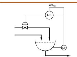
Gain scheduling based on the measurement signal.
