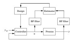
Idea: Track the point on the Nyquist curve identified by the relay autotuner!
