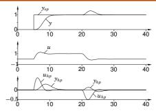
**Set-point changes:**  $|y_{hp}|$  and  $|u_{hp}|$  large, move in the same direction **Load disturbances:**  $|y_{hp}|$  and  $|u_{hp}|$  large, move in opposite direction
