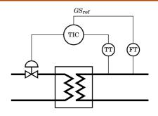
Gain scheduling based on an external signal (the flow).
