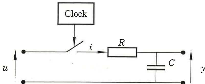
$$m(t) = \begin{cases} 1 & \text{if switch is closed} \\ 0 & \text{if switch is open} \end{cases}$$
